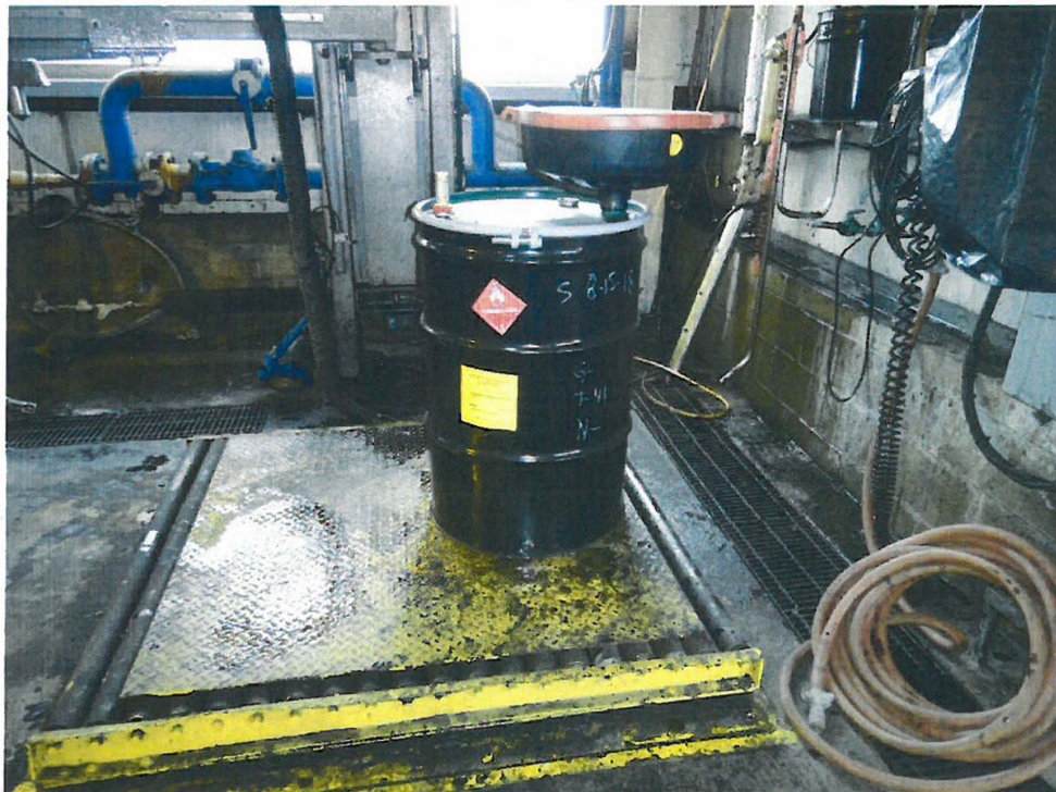
Photo #32: Closed 55-gallon container inside Sanyo Building #3000 (Aclube Unit), labeled as hazardous waste "Aclube Condensate", "D001, U162". Start date 8/15/18. Facility manages container as a Satellite Accumulation Area.
