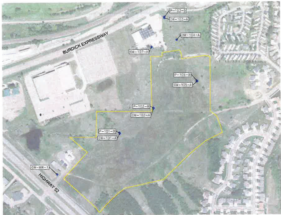
Figure 2.08b.1: Groundwater Monitoring Wells
