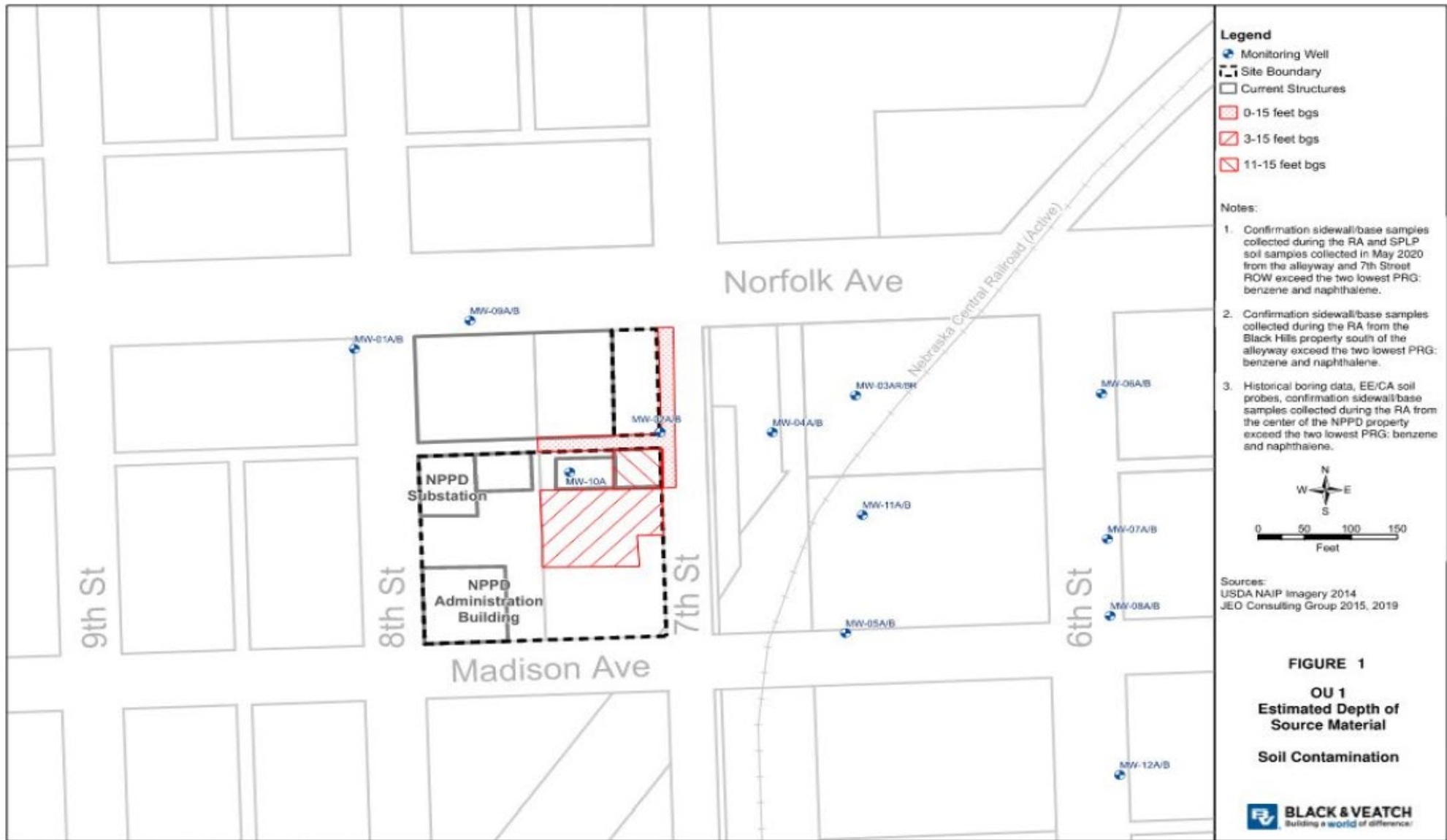
FIGURE 6 - OU 1 Estimated Footprint of Source Material (Remaining Soil Contamination)
