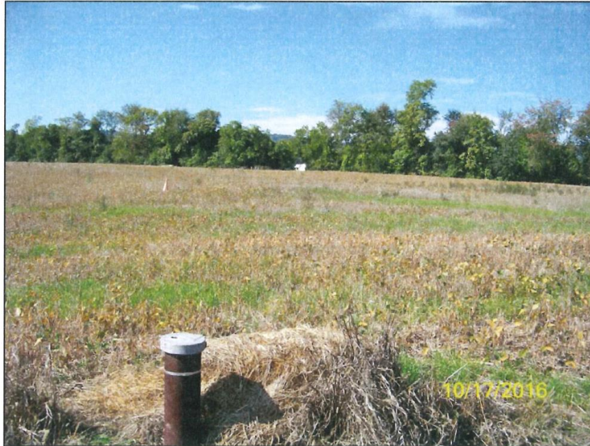
Image 7: CGS-Installed Monitoring Well.
