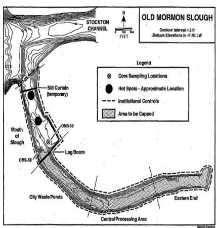
Figure 4.1. Alternative SD-2, In Situ Capping
